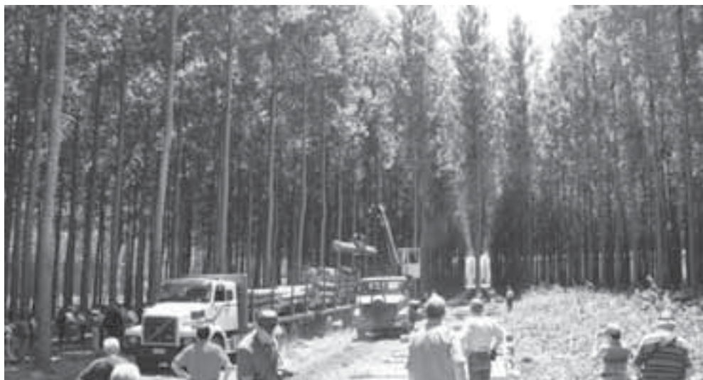
Fig. 5.20. Poplar logs are loaded on to trailers by a crane and transported to the mill. Felling, delimbing and bucking are done manually, by chainsaw crews. Photo courtesy of J. Stanturf.
