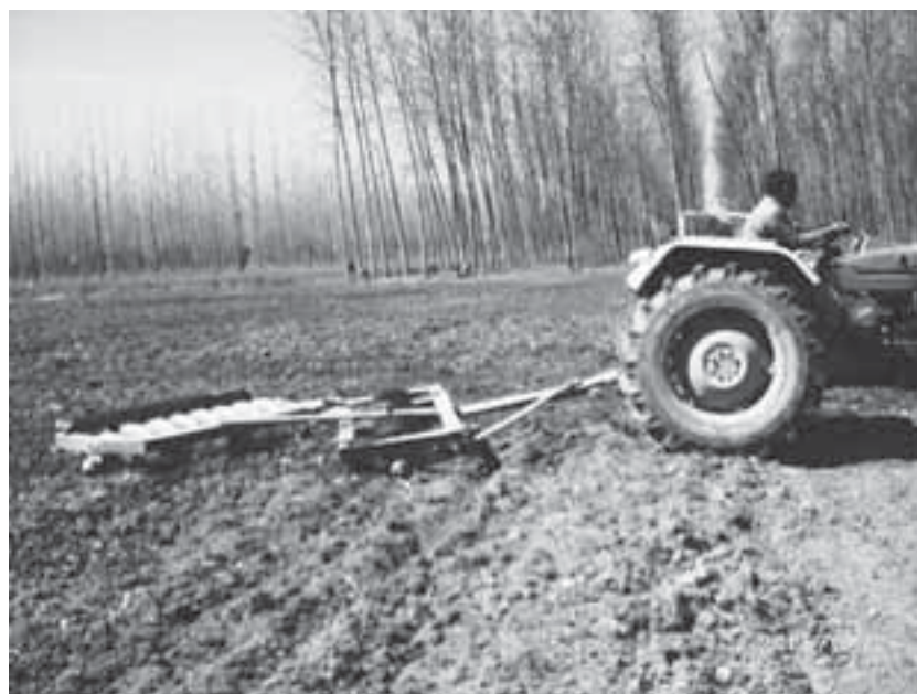
Fig. 5.6. Site preparation by agricultural tractor in India; the operator is cross-disking the site. Older plantations are in the background. Photo courtesy of R.C. Dhiman.
