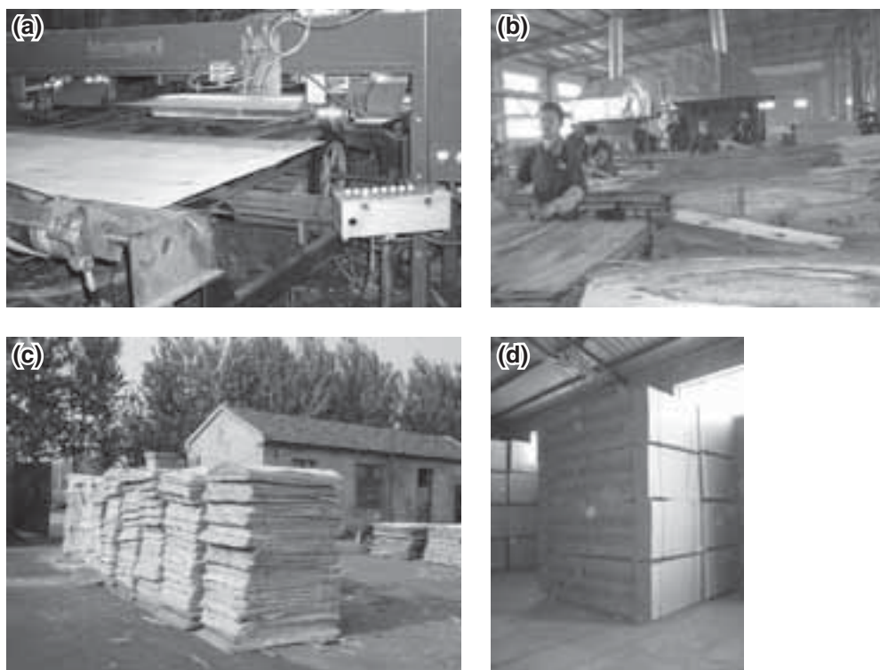
Fig. 10.4. Photographs showing poplar veneer production and products in Canada (a) and China (b–d). (d: 'blockboard' stacks). Photos courtesy of FPInnovations, Forintek Division (a), J. Richardson (b), Nanjing Forestry University (c) and J.G. Isebrands (d).
